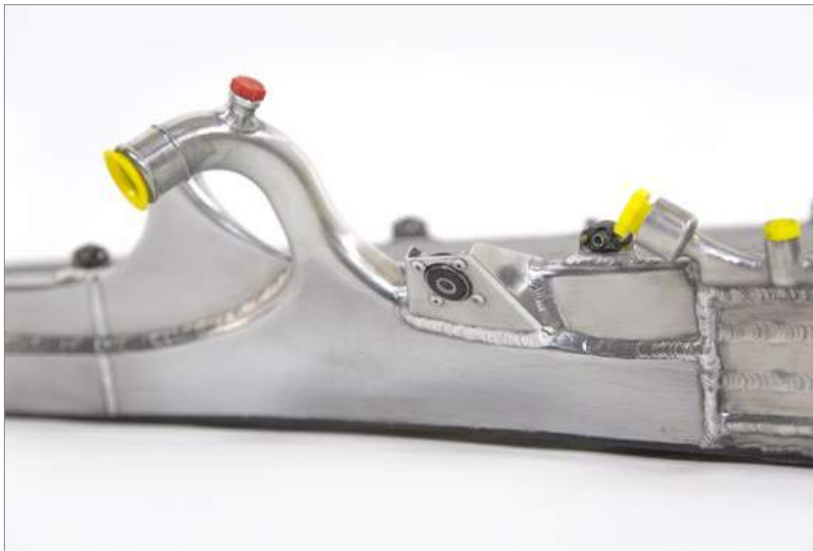
Fig. 13 Detail of the AM inlet tanks
