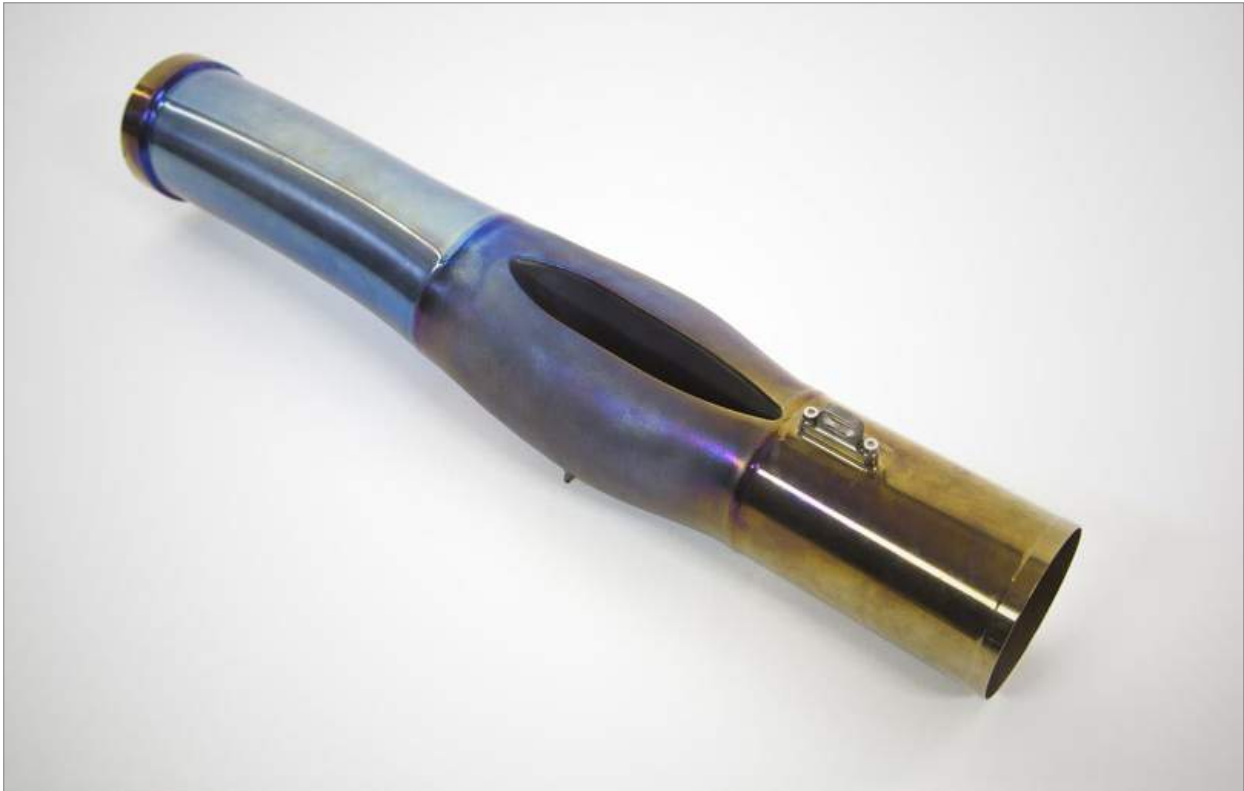
Fig. 10 Titanium race car tailpipe with the central section manufactured by metal Additive Manufacturing
