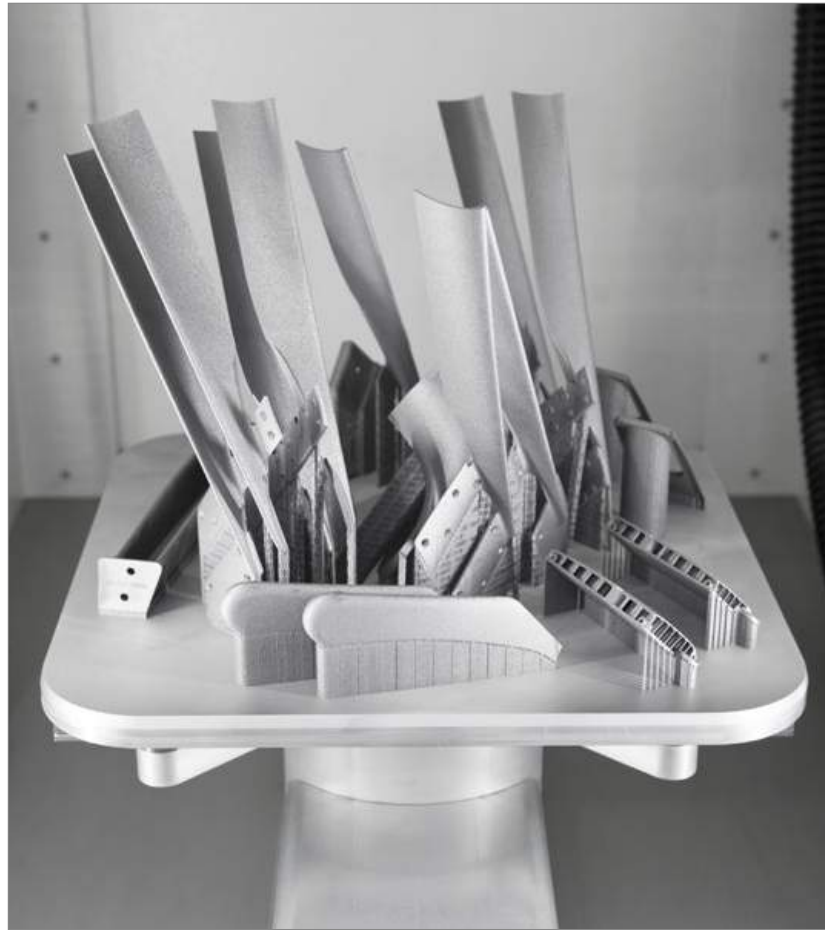
Fig. 6 A build plate with parts for the 60% F1 wind tunnel model and for the 1:1 F1 race car made from AlSi10Mg
