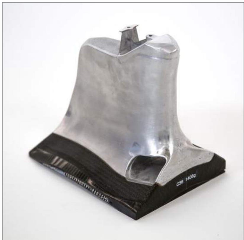
Fig. 11 A Scalmalloy roll hoop, with complex internal structures, which protects the driver in the case of the car inverting
